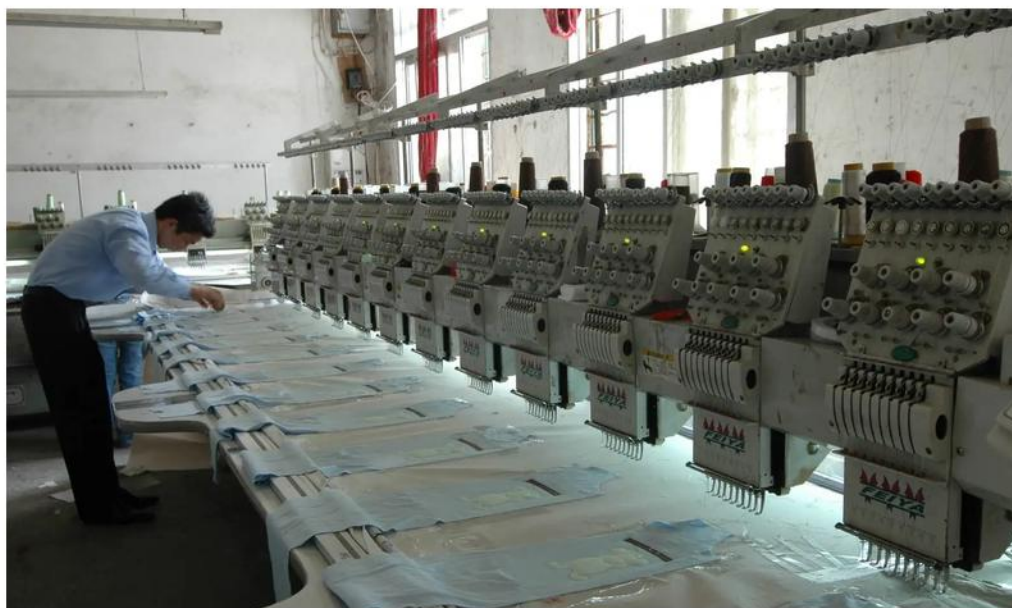
Embroidery floor. Multi-head machines run caps, apron chest logos and bag patches from the same digitised file, which keeps a logo identical across a mixed order.
