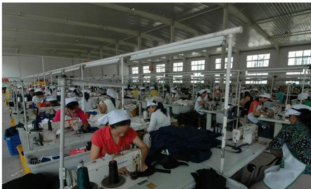
Main sewing floor. Handles, gussets and bindings are set here; handle stitching is the part of a tote that fails first, so it is boxed and bar-tacked rather than straight-stitched.
