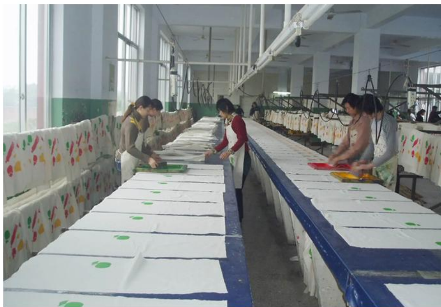
Screen printing line. Flat panels are printed and cured before the bag is assembled, so a large front print stays square and does not distort across a seam.
